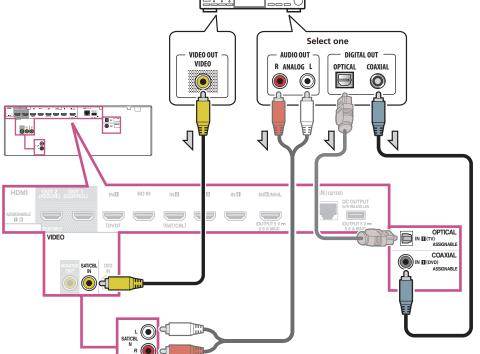
With factory default settings, video from the video cable or component cable will not be output from the HDMI terminal. To output video, you must switch video input to the device connected with the video cable or component cable and set V.CONV to ON (page 69).
